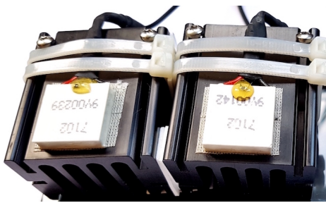
Figure 4: Peltier thermal stimulators (2 x 2cm 2 ) used in the lab study, with heatsinks.
